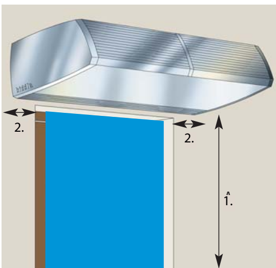
Correct door height and width installation
