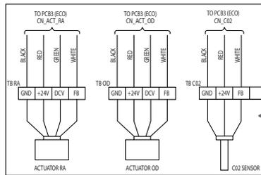
Sticker wiring diagram on the front cover of junction box
