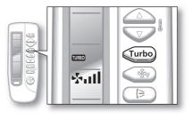
Turbo function is only available in Auto/Cool/Heat mode. If Turbo function is selected in Dry/Fan mode, operating mode changes to Auto.
