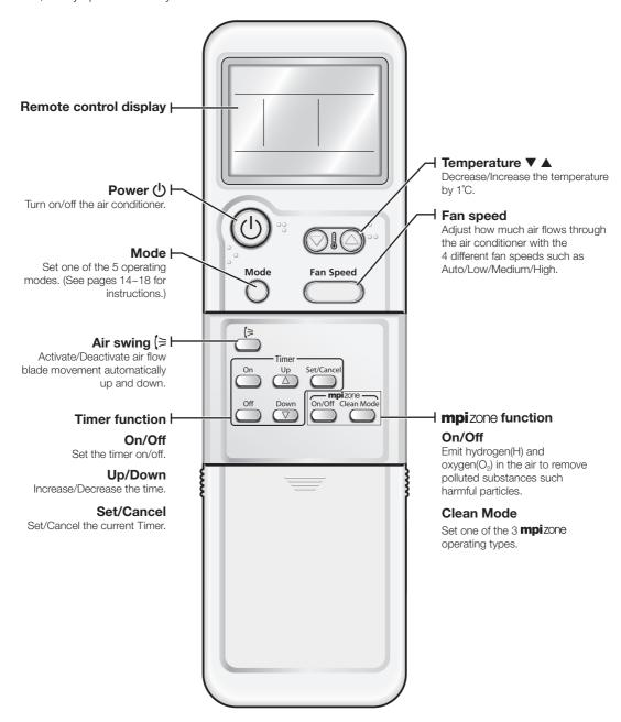
Each time you press the button, a short beep will sound and a transmit indicator appears on the remote control display.
