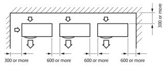
$\displaystyle \pmb{*}$  When 3 sides of the outdoor unit are blocked by the wall
