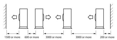
$\*$  When front and rear side of the outdoor unit is towards the wall
