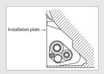
After checking for gas leaks in the system, insulate the pipe, hose and cables. Then place the indoor unit on the installation plate.
