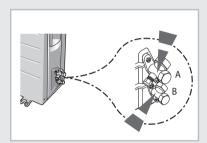
Make sure to check for gas leaks before completing the installation process (connecting the assembly pipe and hose between indoor unit and outdoor unit, insulating the cables, hose and pipe, and fixing the indoor unit to the installation plate)
